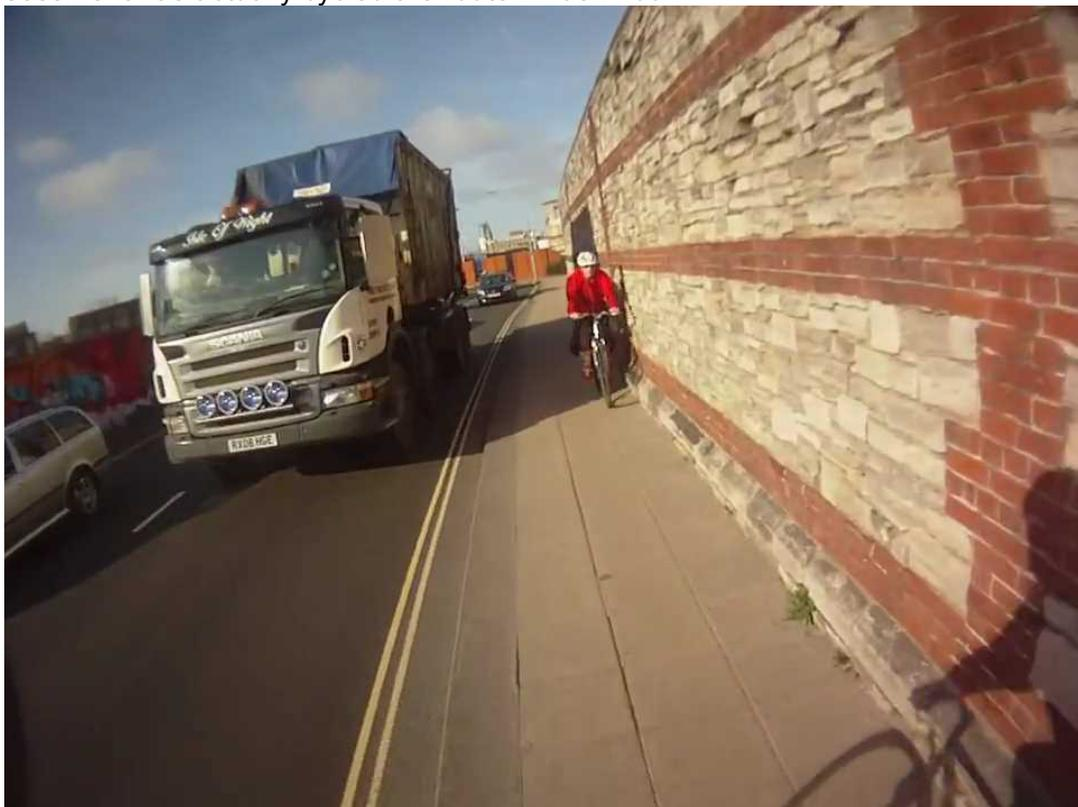
**Hope Street west side narrow (1.5m) shared use pedestrian and cycle path under half DfT minimum recommended width - yet assessed as highest level of cycle and pedestrian safety by WSP**
